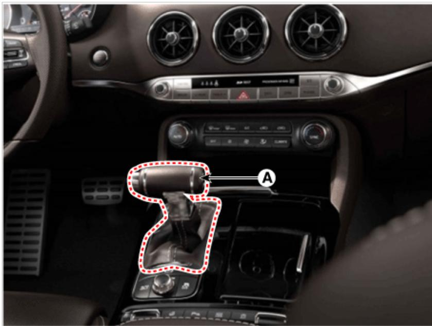
3. Remove the floor console assembly.
