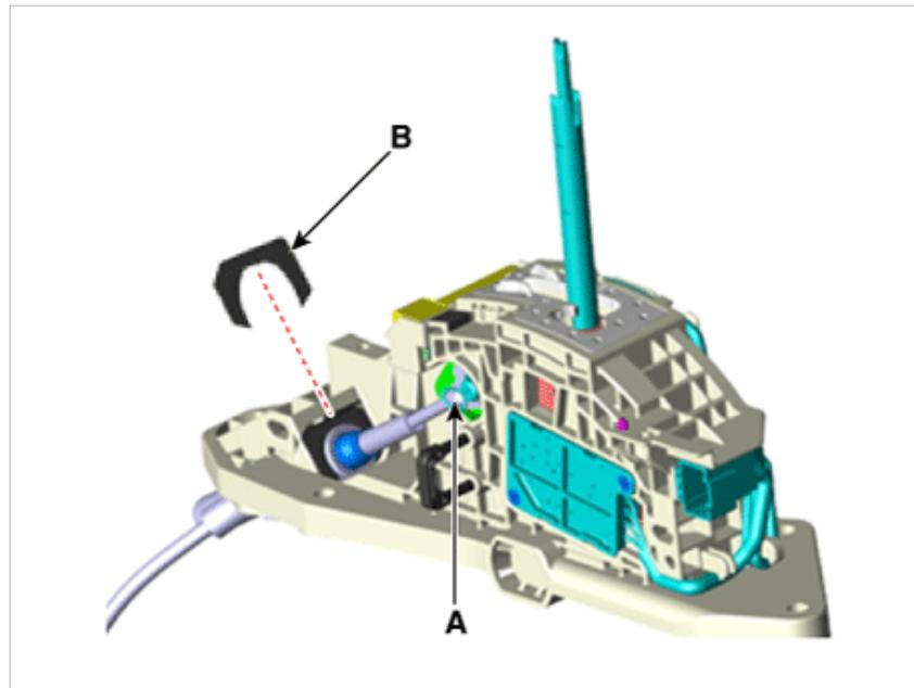
7. Remove the shift cable from the shift lever after loosening the screws (A).
