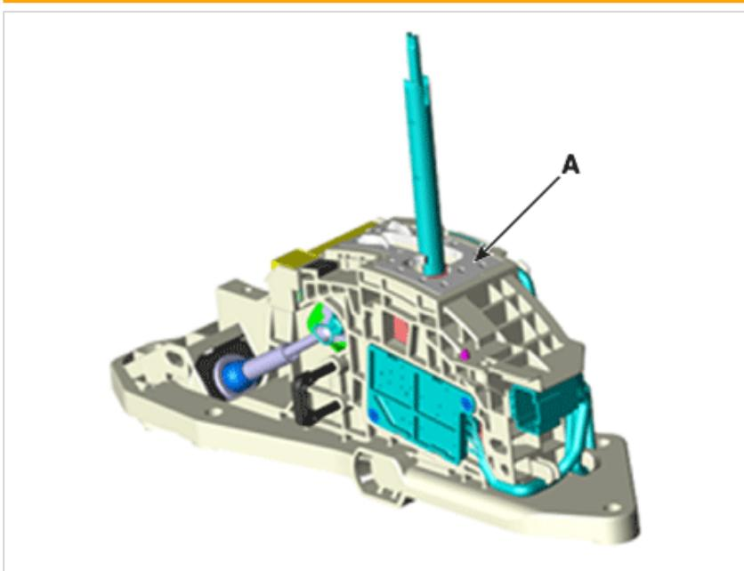
6. Remove the snap pin (A) and shift cable fixing clip (B).
